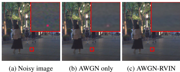
Figure 7: Denoised performance of models trained with AWGN in (b) and mixed AWGN-RVIN in (c). During testing, k = 0 and s = 2 .
