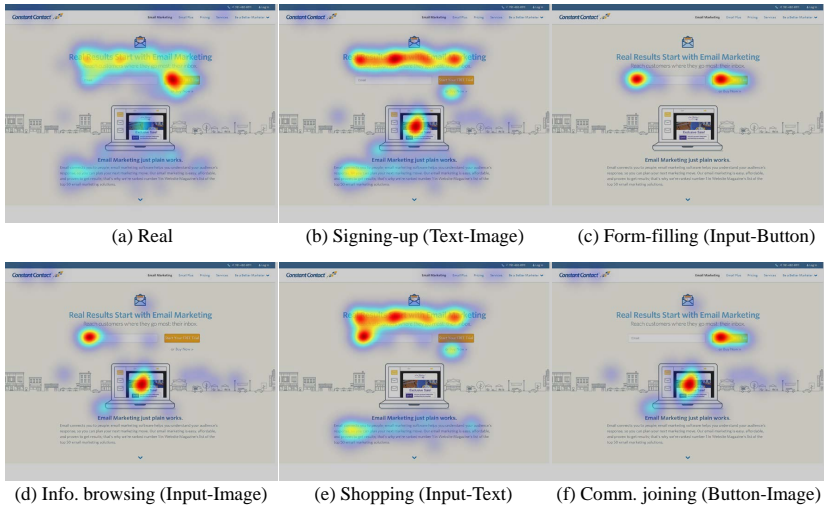
Fig. 5: Synthetic saliency data. (a) Saliency map from the webpage dataset [24]. (b)-(f) Synthesized saliency maps from (a) for 5 different tasks. The corresponding key components of each task are shown in braces.
