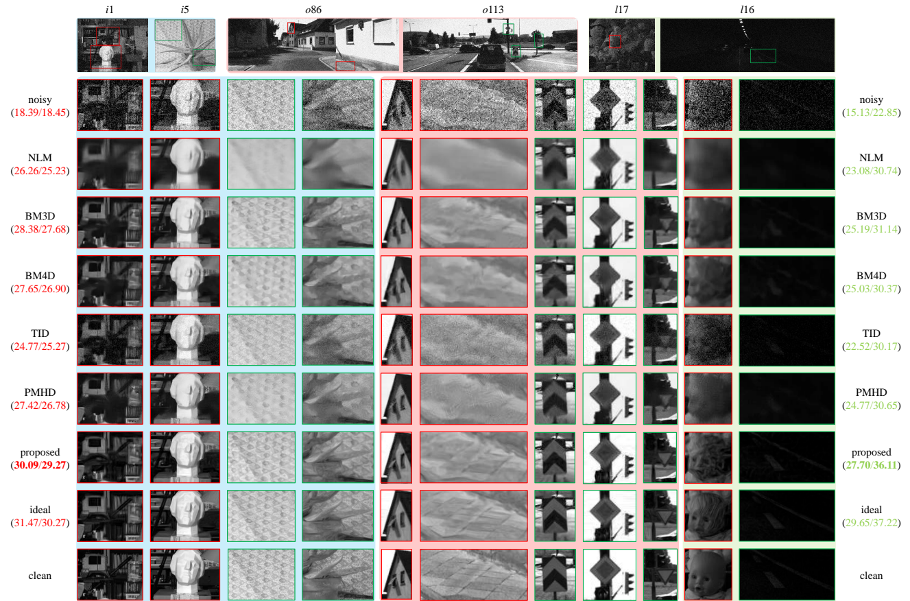
Fig. 14 Qualitative results on the three test sets (indoor (blue), outdoor (red), and low-light (green)) corresponding to the first two, following two, and the last two images in row one). Numbers under each method represent the PSNR values for the outdoor/low-light images.
