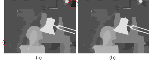
Fig. 4. Disparity maps (a) before and (b) after dark region refinement.
