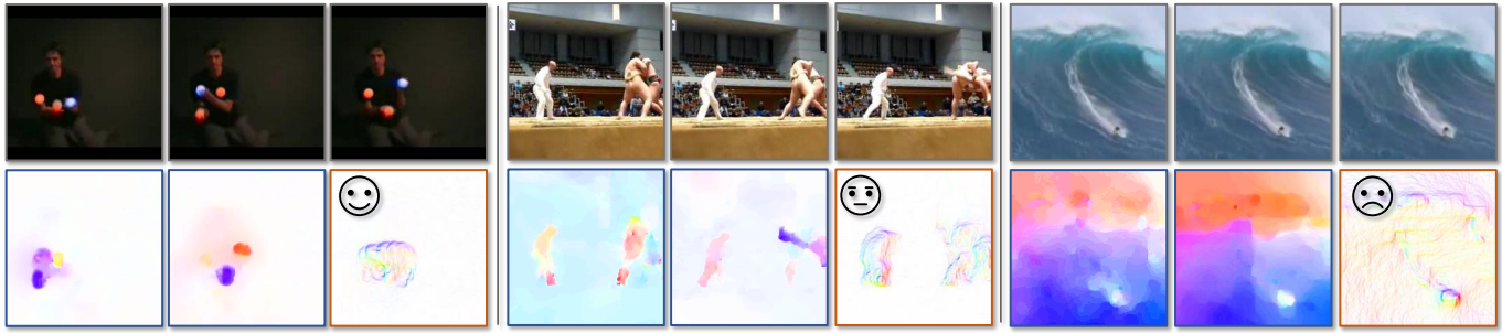
Fig. 9. Three video samples of the curriculum learning strategy. From left to right, the difficulty to predict the motion statistical labels of each video clip is increasing. For each sample, the top three images are the first, middle, and last frames of a video clip. In the bottom row, the first two images are the corresponding optical flows and the last image is the summarized motion boundaries M_u/M_v with the maximum magnitude sum.
